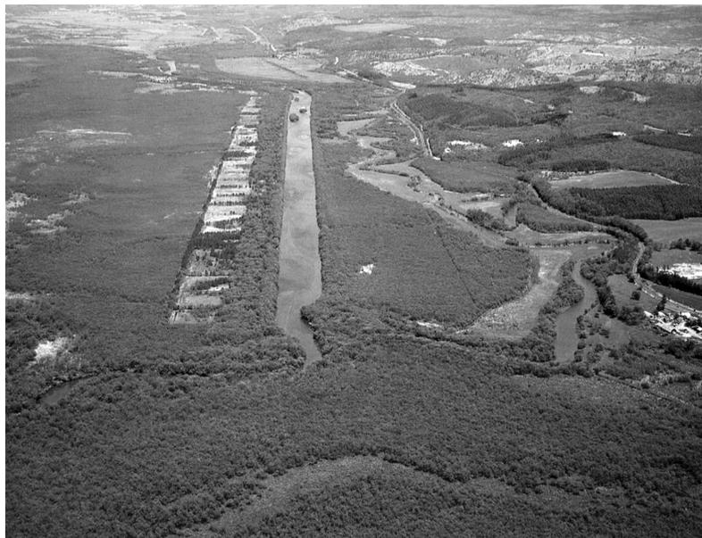
**Fig. 7.** Re-meandering project in Kushiro River. The central channelized section is planned be reconnected with the old meandering reach (right side of the picture).
